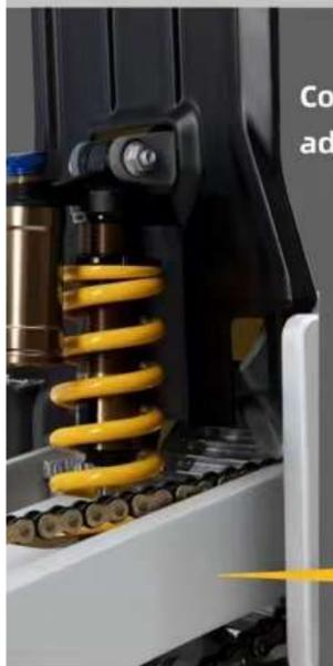
Compression, rebound multi - level adjustable rear suspension system
